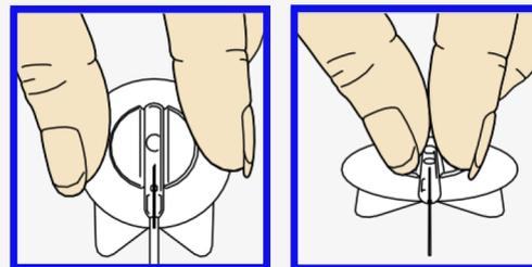
Hold infusion set insertion piece by flipping the plastic wings upwards and pressing them together.
