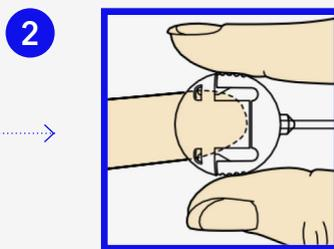
2 Press the edges of the set release connector. With the other hand, pull the cap off.
