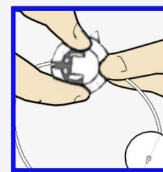
3 Slide the set release connector into the set connector.
