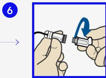
6 Twist the plunger counter-clockwise to loosen and remove.
