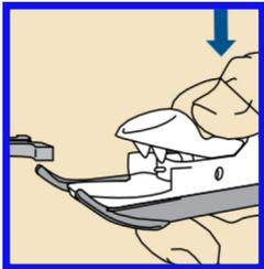
Use thumb to press down on the Lock & Release handle of theserter.
