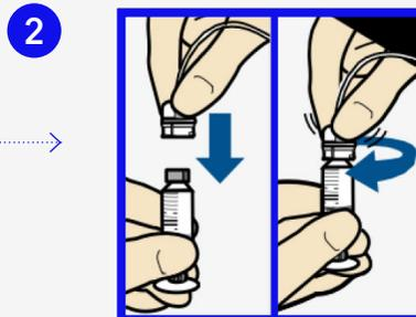
2 Gently push the tubing connector onto reservoir. Turn clockwise until locked. You will hear a click.
