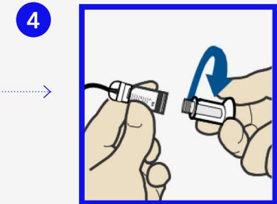
4 Twist the plunger counter-clockwise to loosen and remove.
