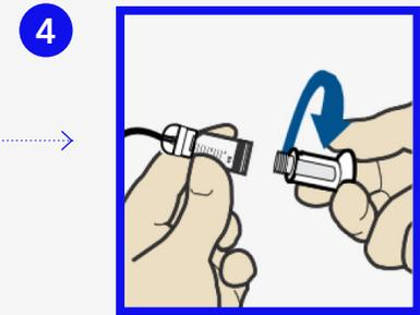
Twist the plunger counter-clockwise to loosen and remove.
