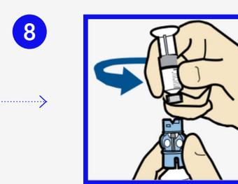
To avoid getting insulin on the top of the reservoir, turn vial over so it is upright. Hold transfer guard and turn reservoir counter-clockwise and remove from transfer guard.
