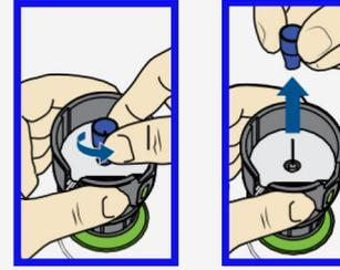
Turn to loosen needle guard and pull.
