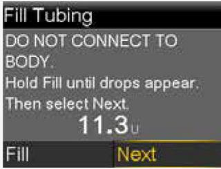
Select **Load** and keep holding **O**.      When you see this screen, select **Next**.      Select **Fill** and keep holding **O** until you see drops at the end of tubing, then let go.      Drops at end of tubing.      After you see drops, press **>** and select **Next**.
