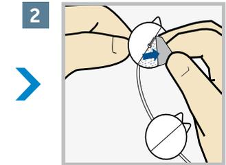
2 Peel off both pieces of the paper backing from the insertion piece.
