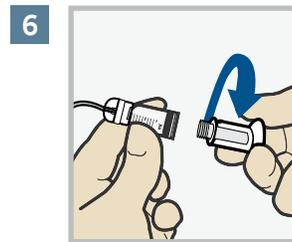
6 Twist plunger counter-clockwise to loosen and remove.
