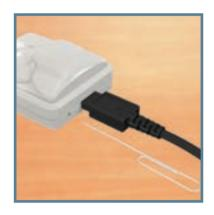
Reset the iPro2 recorder by inserting a paper clip into the white docking station. See page 3 for pictures.
