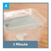
**4.** Submerge recorder in the solution for at least 1 minute.
