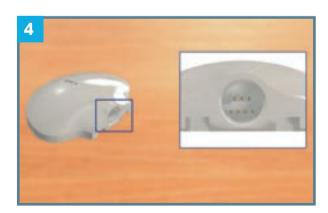
4. Be sure to check and make sure no blood is inside the recorder before inserting the cleaning plug in the next step. Important: If there is blood inside the recorder, throw it in a sharps container.
