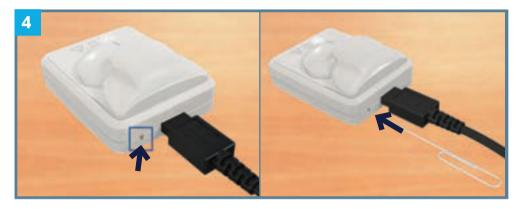
4. The recorder is delivered in sleep mode to preserve battery life and it must be activated. Find the small hole on the back of the docking station. Use the end of a paper-clip to push in about 3mm and release.
