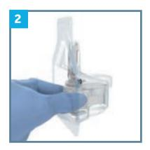
2. Hold the plastic pedestal. Remove the sensor and put it on a flat surface.
