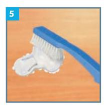
**5.** Remove recorder from solution and lightly brush entire surface.
