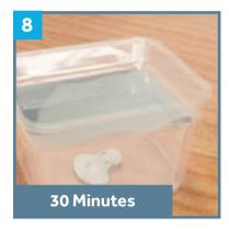
8. Submerge recorder in the bleach solution for 30 minutes.
