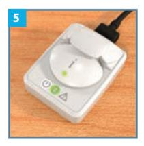
5. The white docking station power light will flash. After a few seconds the green light on the iPro2 recorder will flash green.
