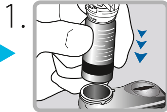
Place reservoir into pump.
