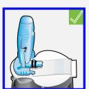
Tuck the adhesive tab. Make sure that the sensor's adhesive tab is tucked under the sensor connector and snaps.
