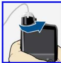
Remove the used reservoir from the pump.
