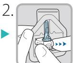
Remove the sensor with attached pedestal by holding the pedestal. Place the sensor/pedestal on a clean, flat surface (such as a table).
